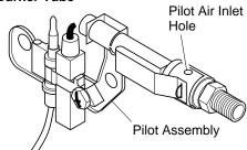
Figure 29 - Pilot Inlet Air Hole
